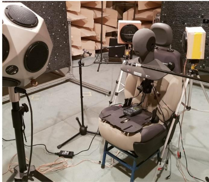
**Figure 4.** ANC tests under semi-anechoic conditions.
